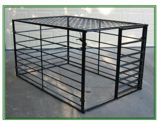
This stock rack has a 3/4" square tubing frame and  $\frac{1}{2}$ " rails and is a light weight rack, yet strong enough for your toughest rams and bucks. For easy assembly it is made in 4 pin together section or as one welded unit.
